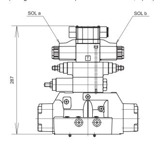
With MT-02W-60 (type W) (Hexagon socket head cap bolts used: M5 × 85, 4 pcs.)
